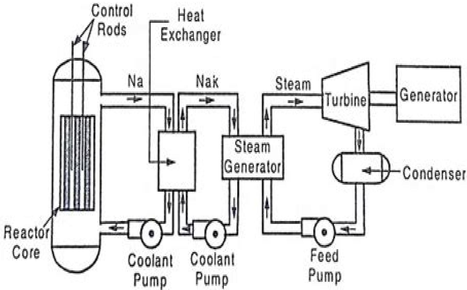
Fig:3.12 Liquid Metal Cooled Reactor
