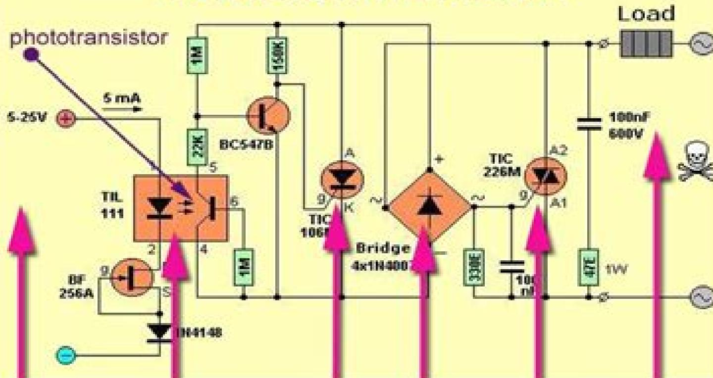
controlled AC source to load (motor lights)
