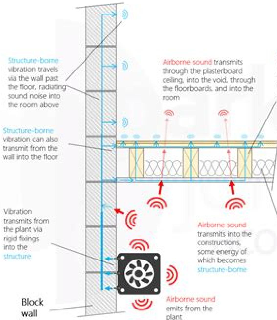
Structure-borne sound transmits between the ceiling and floorboard via rigid connections in the form of timber floor joists, radiating sound into the room above.
