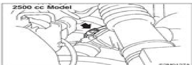
3) Disconnect rear oxygen sensor connector.
