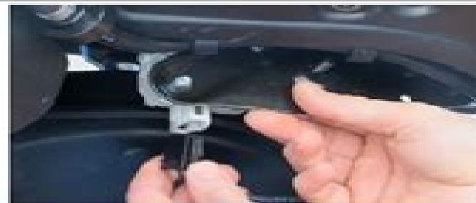
Connect the cable to the saddle's lock.
