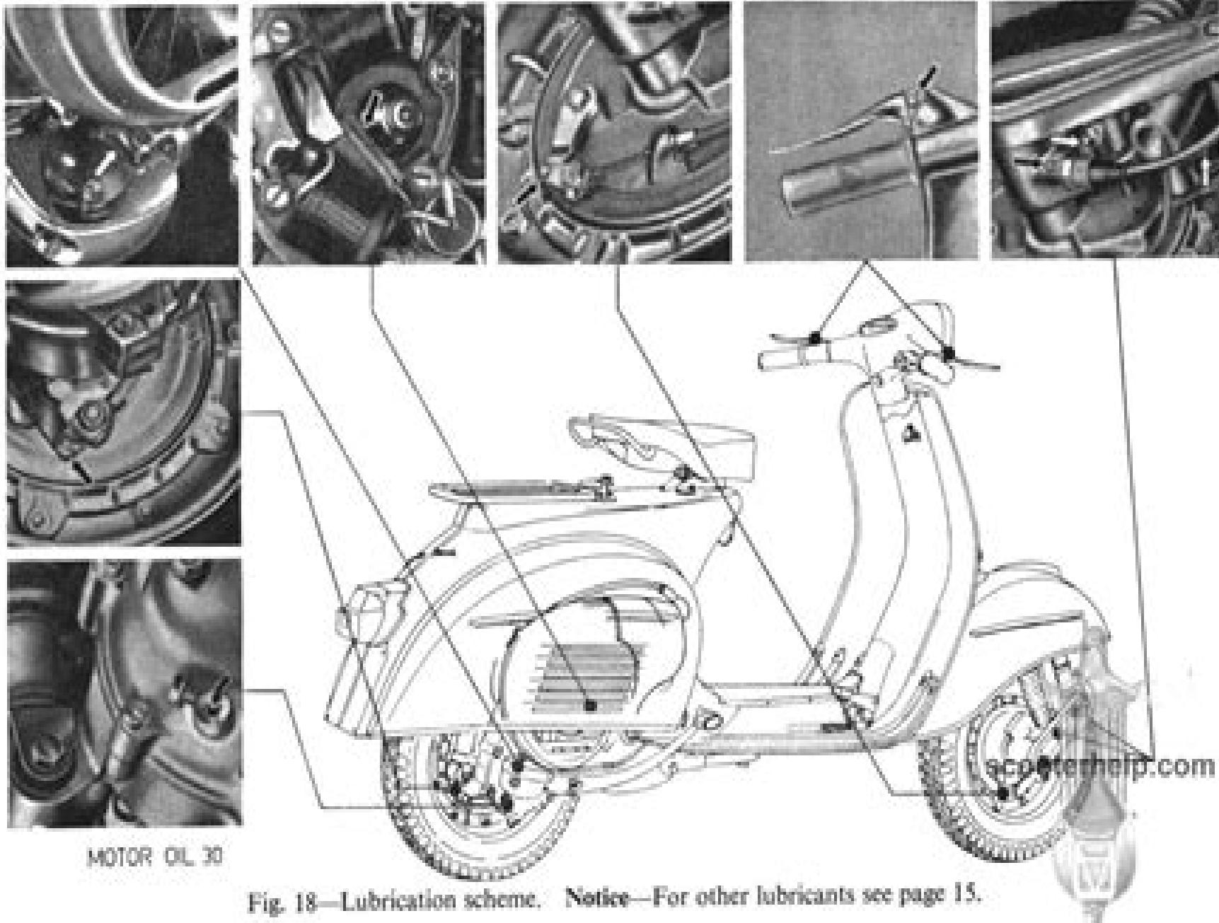
Fig. 18—Lubrication scheme. Notice—For other lubricants see page 15.
