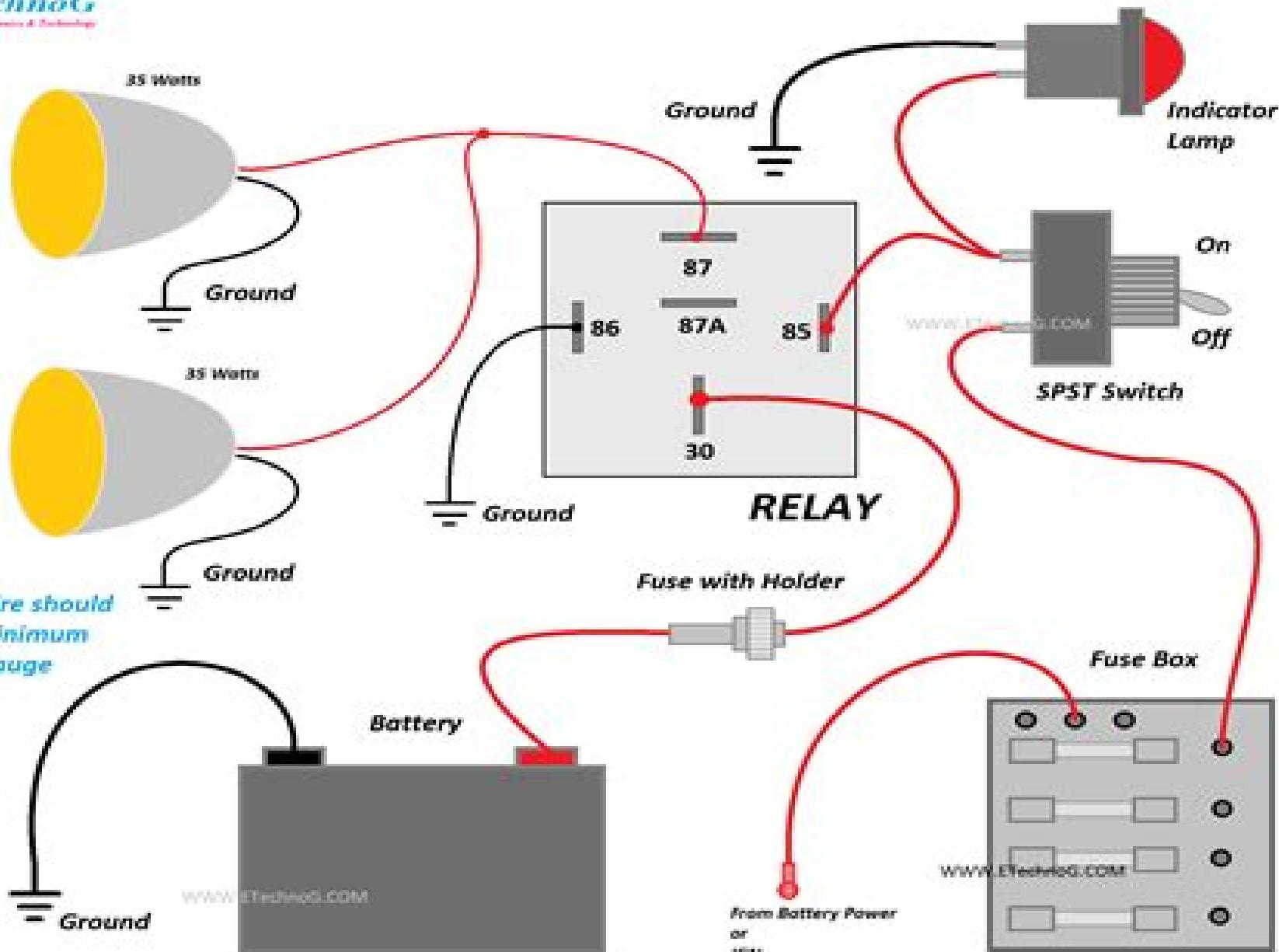
**Fog Light Wiring and Connection Diagram with Relay and Switch**
