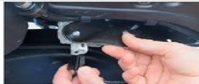
Connect the cable to the saddle's lock.
