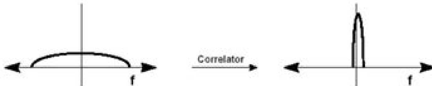
Figure 5b Received Signal is Correlated with PN to Recover Data and Reject Interference
