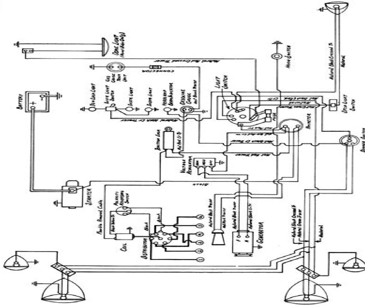
Fig. 60—Passenger Car Wiring Diagram
