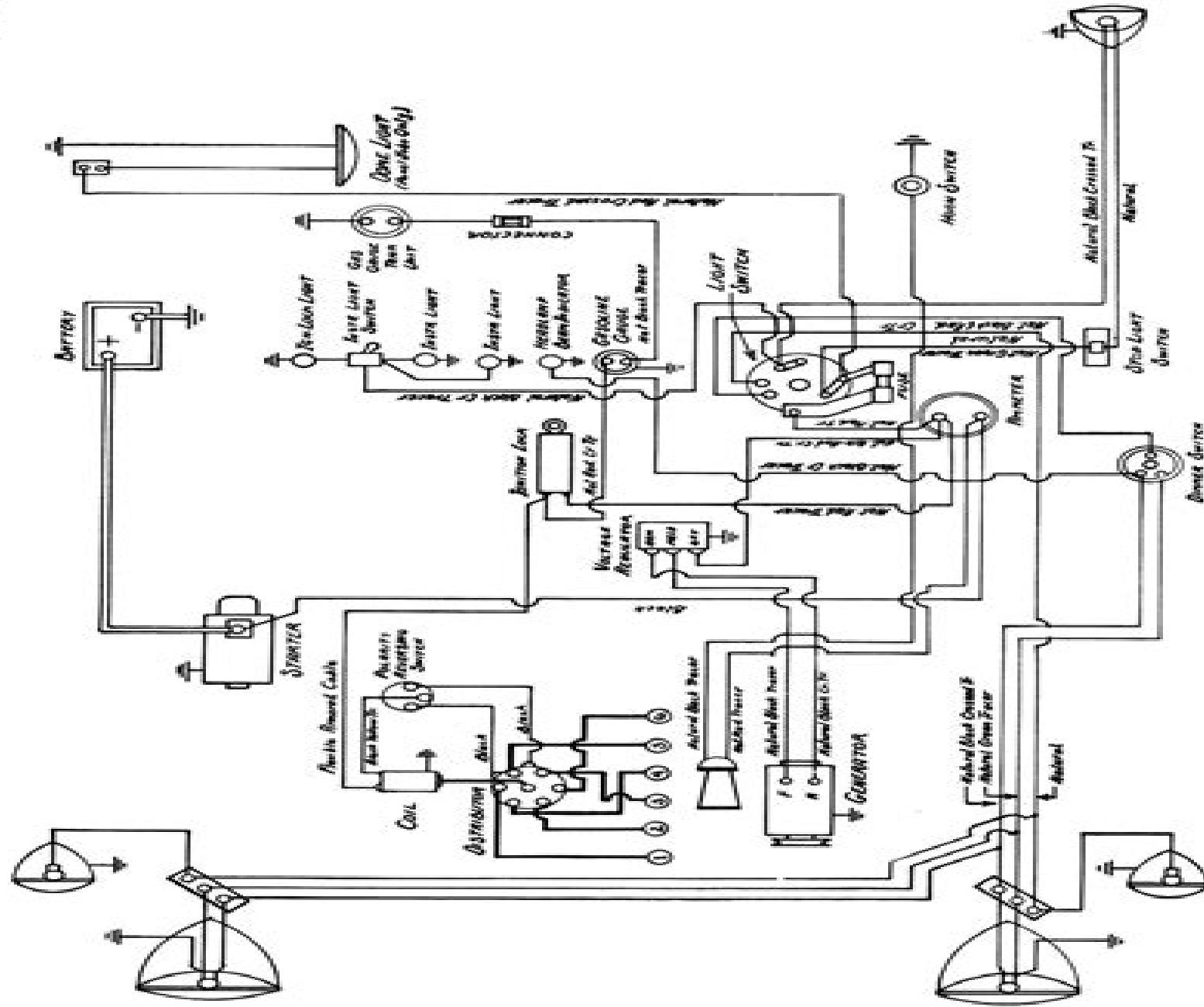
Fig. 60—Passenger Car Wiring Diagram
