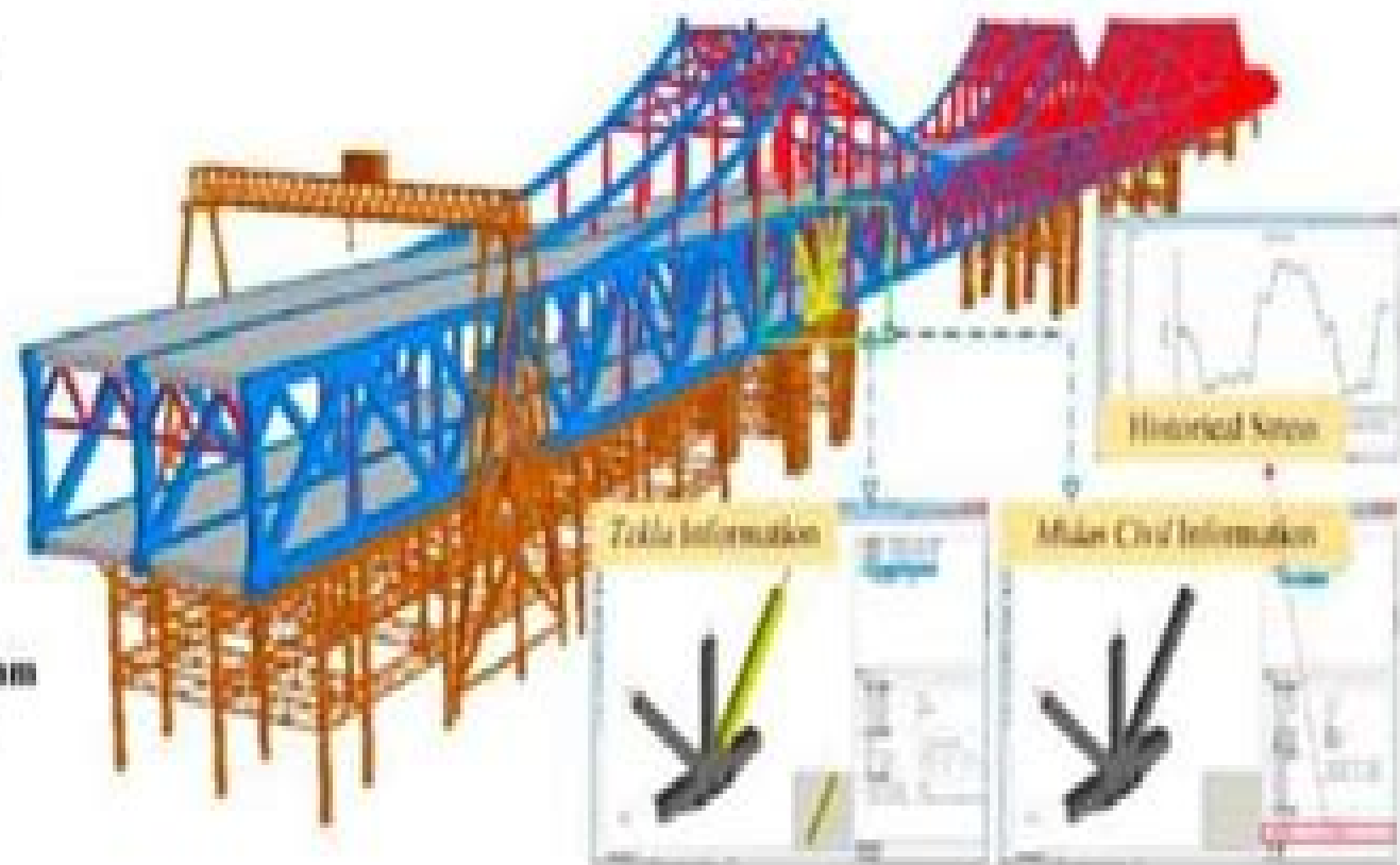
Different case models' stress nephogram
