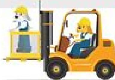
If forklift is being used to elevate a worker, make sure worker uses restraints and is elevated using a platform or cage.
