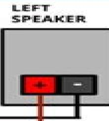
For basic stereo wiring, connect one (marked) wire as the positive and one as negative. For more speakers, repeat the same.
