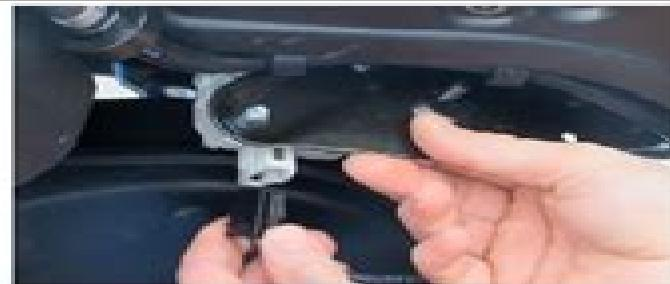
Connect the cable to the saddle's lock.
