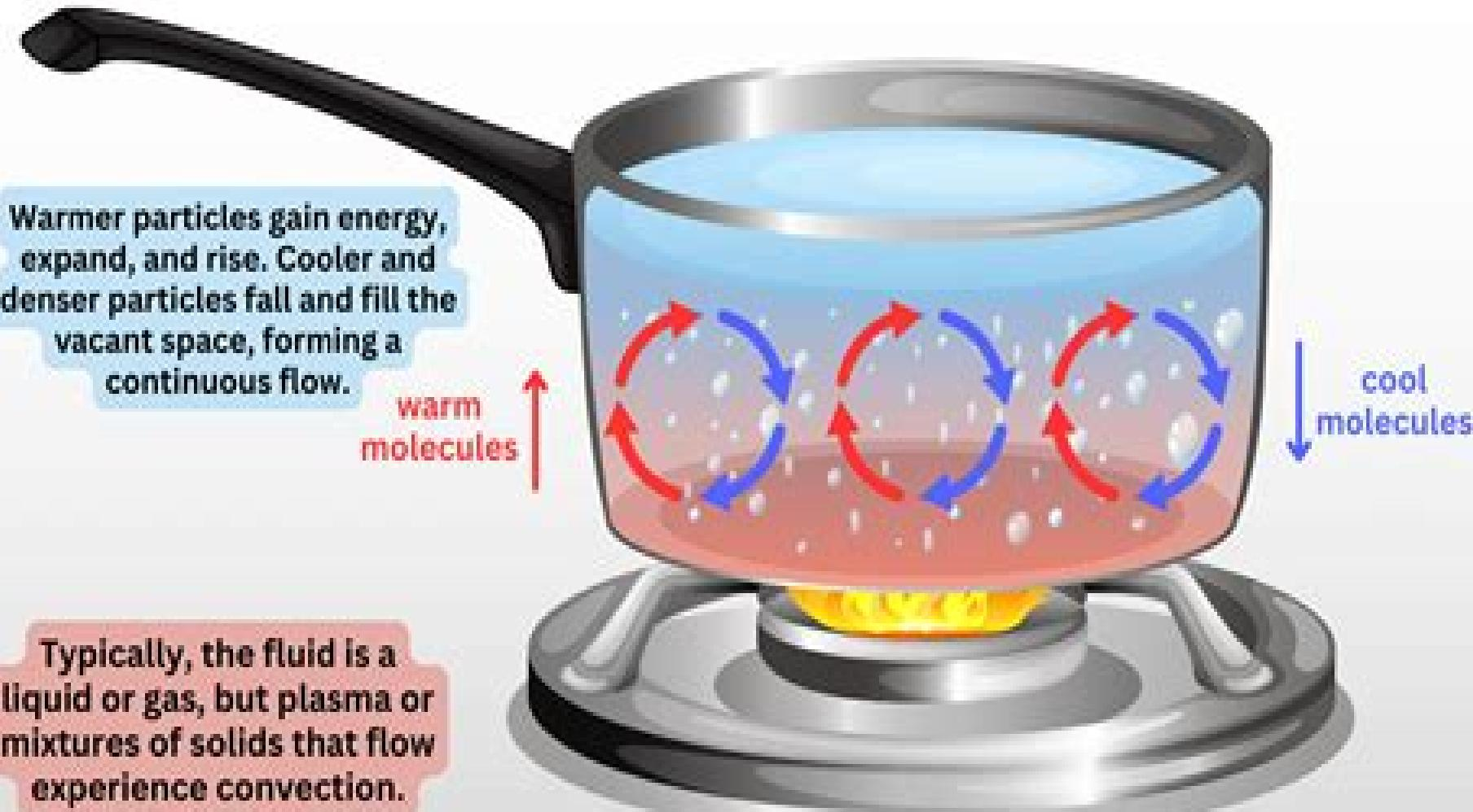
Typically, the fluid is a liquid or gas, but plasma or mixtures of solids that flow experience convection.
