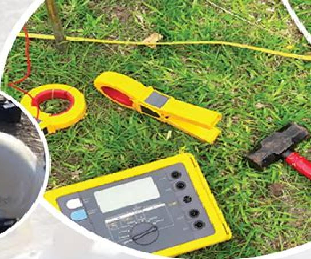
**Soil resistivity test** determine low resistivity zone for design of grounding system, Earthing systems. On the basis of field data collected and earthing test report generated type of grounding design system i.e Electrode earthing , Chemical Earthing can be determine .
