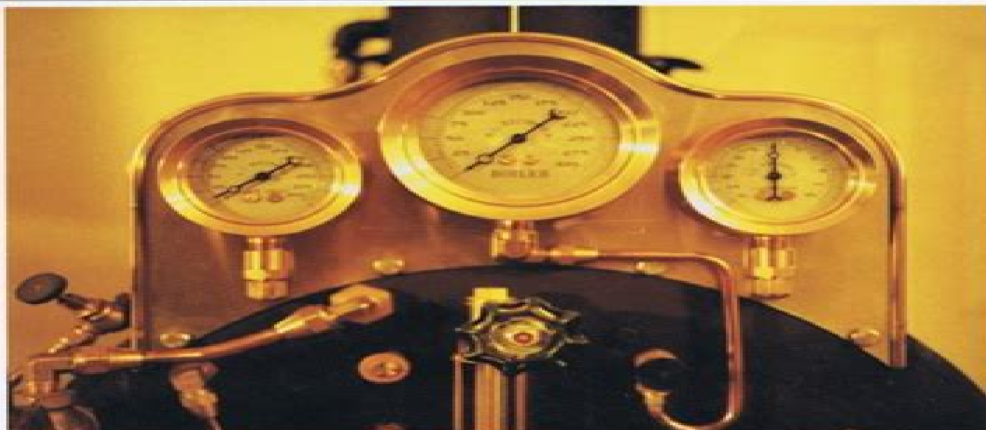
Boiler face and gage board for H. K. Anderson's RECIPROCA . See page II-30-1
