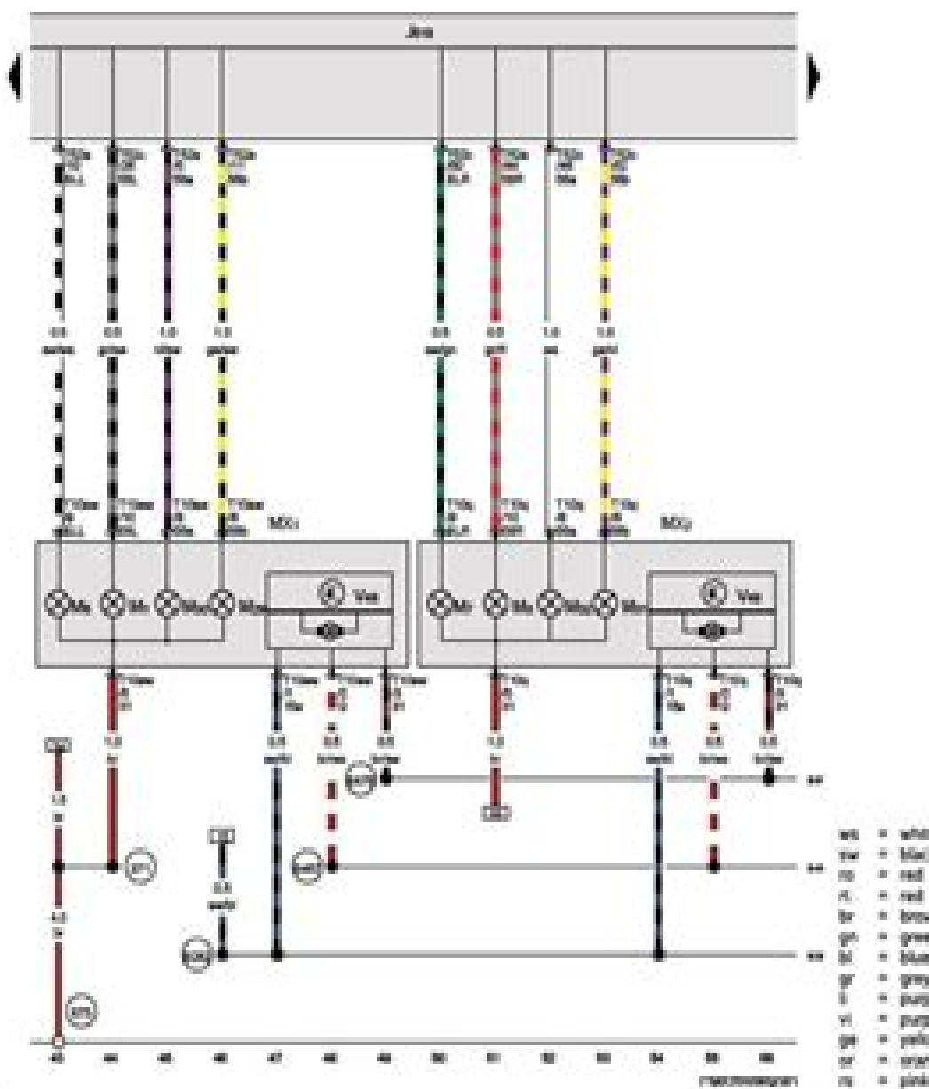
Onboard supply control unit, Front left headlight, Front right headlight
