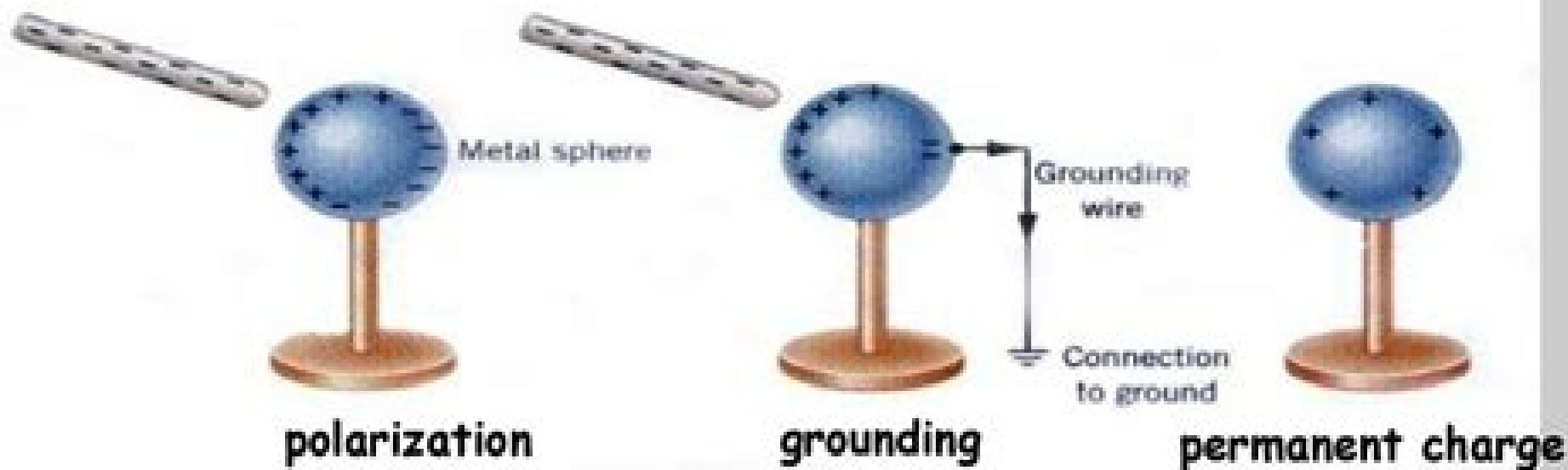
The rod does not touch the sphere. It pushes electrons out of the back side of the sphere and down the wire to **ground**. The ground wire is disconnected to prevent the return of the electrons from ground, then the rod is removed.
