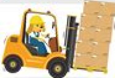
Use seat belts, assigned seats and no joy riding while operating. When work is complete, engage brakes, lower forks and turn off controls.
