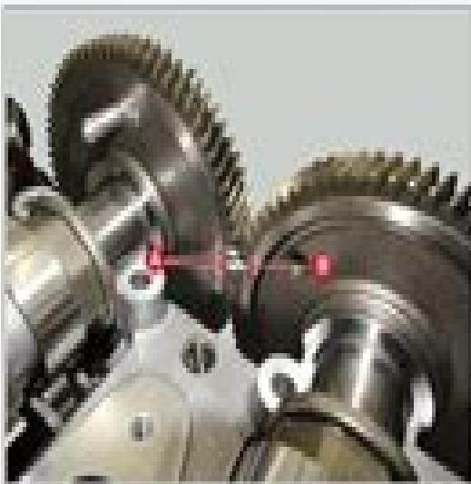
10. Rotate the crankshaft counter-clockwise by 30° to align the yellow mark on the crankshaft sprocket with the assembly surface (horizontal surface) of the cylinder block and bearing cap (0° 1 cylinder piston compression TDC position).
