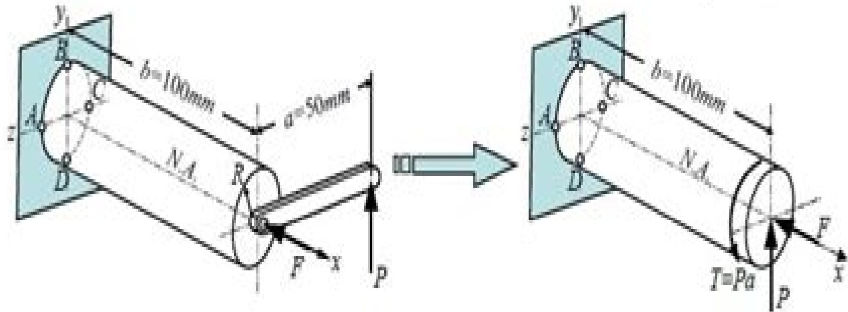
Step 0: Determine the geometrical properties of cross section:
